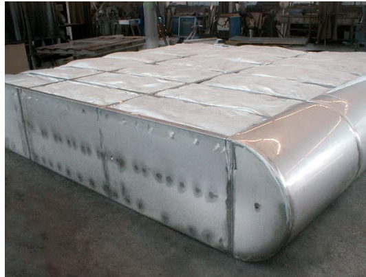
Exhaust silencer with pillow infill.
