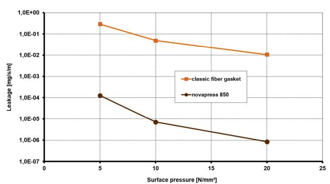
Leakage performance dimensions 92 x 49 x 1 mm, 10 bar Helium, 20°C
