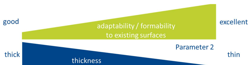
Picture 1: Relation between material thickness and flexibility
