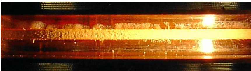
picture 5 gap with spray after 30 sec. 6 bar (87 psi)
