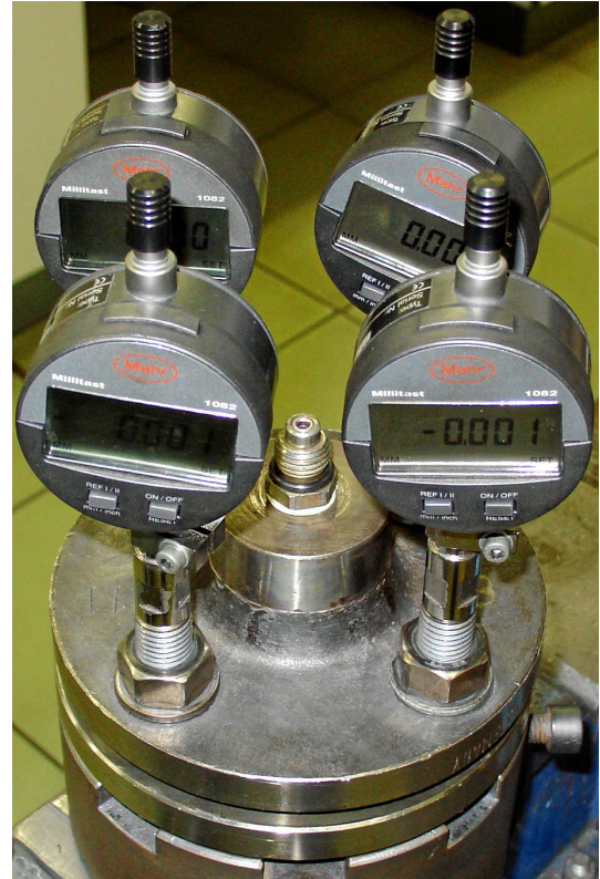
Picture 3 test flange assembled
