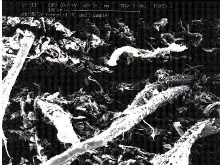
under the electron scan microscope graphite flakes with Kevlar fibres
